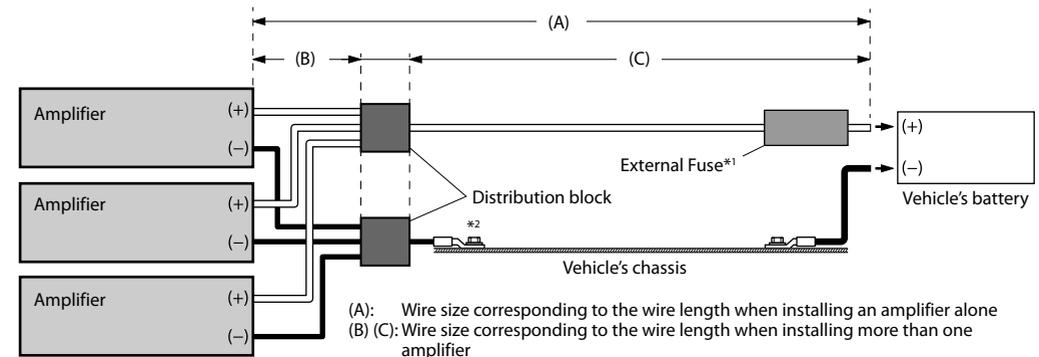
\*1 Be sure to add an External Fuse (e.g. Fuse Block, Circuit Breaker) with the battery lead as close as possible to the battery's positive (+) terminal.
